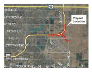
The planned roadway improvements consist of Portland cement concrete pavement, except for the detour roads and the transitions along Ellsworth Road from new construction to existing asphalt concrete pavement. The improvements associated with SR 202L will receive a rubberized asphalt overlay.
