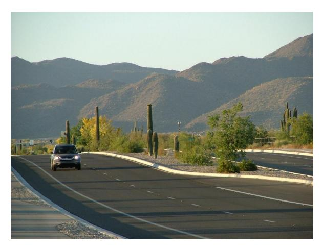
Twin Peaks Road extends nearly three miles, from Interstate 10 to the Tangerine Road. Ninety percent of the road was constructed through an undeveloped Sonoran Desert landscape with a small portion of the project consisting of the widening and reconstruction of an existing street. The roadway cross-section consists of two travel lanes and a bike lane in each direction, a center median, a walkway on the east side, and a shared-use path on the west side.
