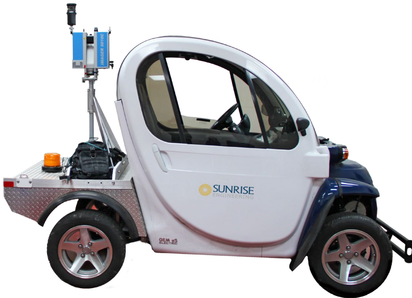
P3D PROSCAN PLATFORM USES THE 5010C FOR INDOOR/OUTDOOR MOBILE APPLICATIONS
